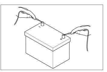
Figure 35. Check Battery Voltage
