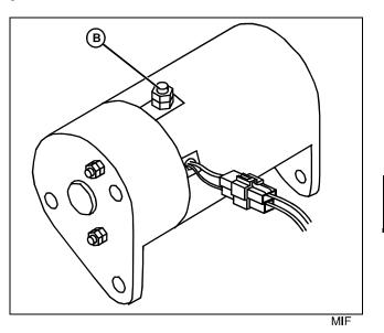
(2) Is battery voltage present at G2 starting motor/ generator - F2 terminal, 240 Red wire (B) with starting motor turning engine?
