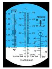
Figure 9. Uncalibrated **Refractometer Scale**
