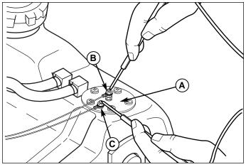
Figure 53. Fuel Level Sensor Volt Test A. Sensor C. Ground Terminal B. Signal Terminal
