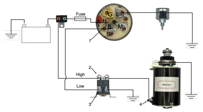
Figure 7. Starter Circuit with Fuel Solenoid
