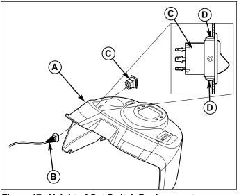
Figure 17. Height of Cut Switch ReplacementA DashboardC. Height of Cut SwitchB. Wire HarnessD. Locking Tabs
