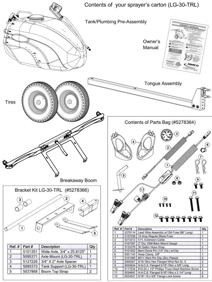
Your tank comes pre-assembled with the pump, manifold, bypass, intake assembly, lid w/lanyard, handgun, handgun hose, handgun hose quick connect and loom clamp already attached.
