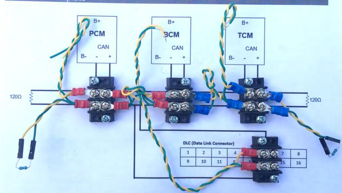
Figure 5. CAN Circuit Assembly
