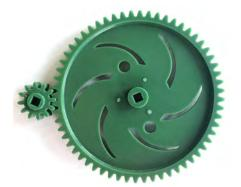
**Ranking: 2** Drive Gear = 12 teeth Driven Gear = 36 teeth
