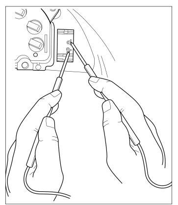
Figure 52. Testing Driving Light Switch
