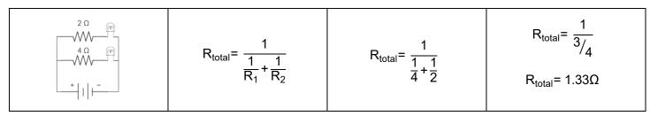
Figure 3. Parallel Circuit
