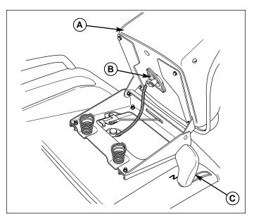
Figure 49. Seat Switch Safety System A. Seat C. Cruise Control Lever B. Seat Switch
