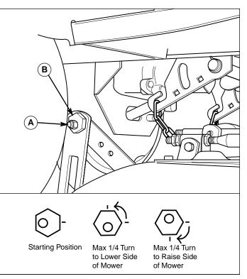
Figure 8. Side-to-Side AdjustmentA. Outside NutB. Eccentric Nut
