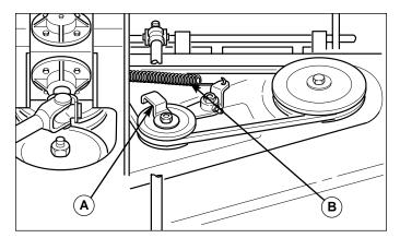
Figure 10. Pulley Stop Position A. Pulley Stop B. Idler Arm Tension Spring
