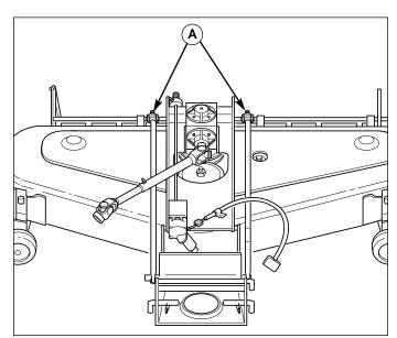
Figure 9. Front to Back Leveling A. Jam Nuts
