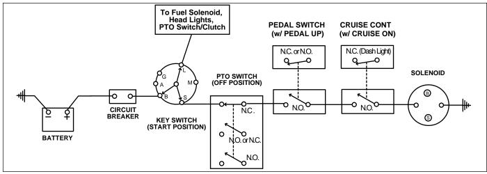
Figure 8. Typical Cranking Linear Circuit Diagram (All Models)
