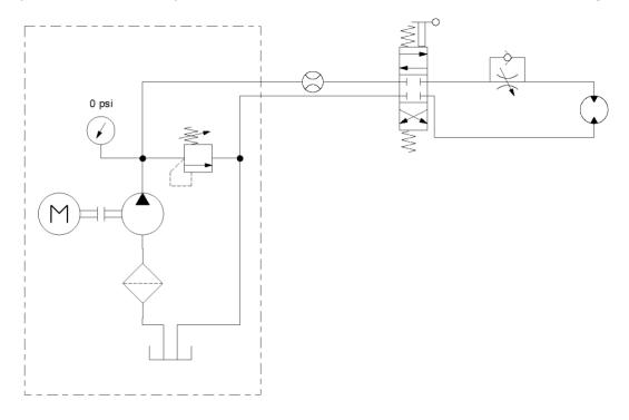
Figure 5. Flow Control Schematic
