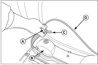
Figure 25. Headlight Lamp Removal and ReplacementA. SocketC. Halogen Bulb
