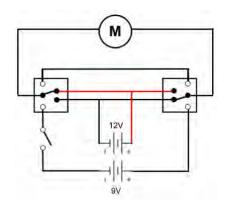
Figure 1. Motor Direction Control
