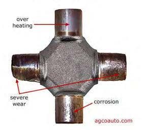
Figure 3. Universal Joint Failures
