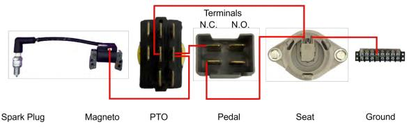
Figure 1. Circuit Schematic
