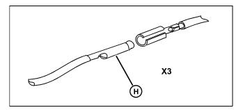
(7) Is there continuity between X3 connector (H) and magneto run relay, with no continuity to ground?
