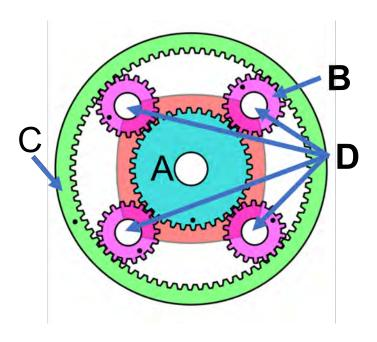
Figure 1. Planetary Gear
