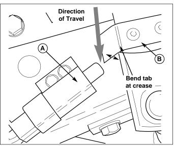
Figure 2. Brake Switch Adjustment A. Brake Switch B. Tab
