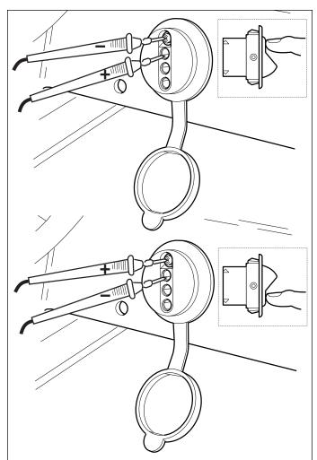
Figure 46. Testing Accessary Connector
