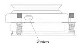
Figure 2. Window View of Air Gap
