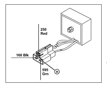
(6) Is there greater than 0 volts and less than 12.0 volts at the voltage regulator 595 Grn wire connector (H)?
