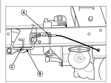
Figure 4. Differential Lock Cable Adjustment
