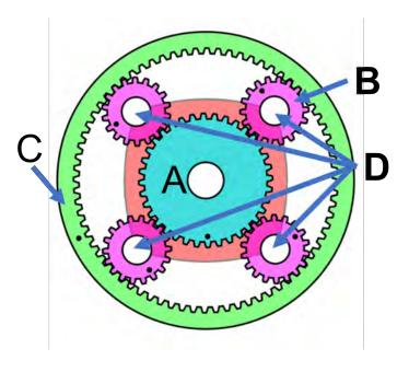
**Figure 1. Planetary Gear**
