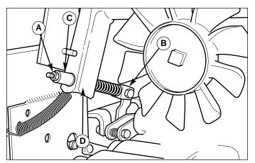
Figure 1. Brake Linkage Adjustment
