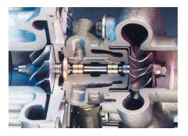
Figure 2. Turbocharger
