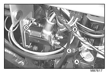
8. Connect VOM to negative (–) battery terminal (A) and terminal (B) of starter solenoid. Check for battery voltage.
