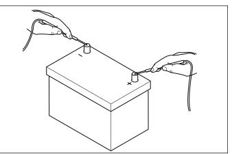
Figure 36. Check Battery Voltage
