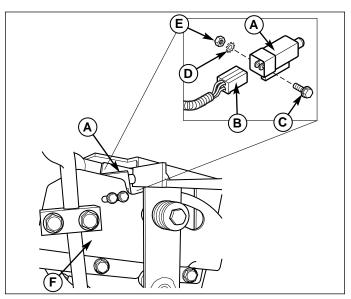
Figure 24. Cruise Switch Removal and Replacement D. Washer
