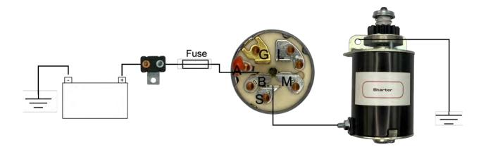
Figure 6. Starter Circuit without Solenoid
