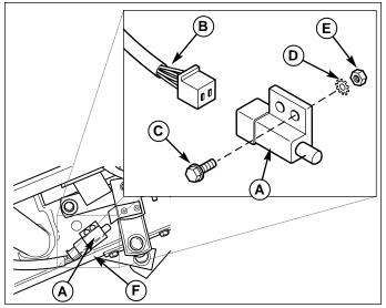
Figure 23. Brake Pedal Switch Removal and Replacement A. Switch **D.** Washer
