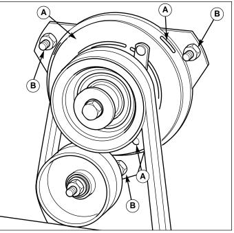
Figure 6. Front PTO Adjustment A. Slots B. Nuts
