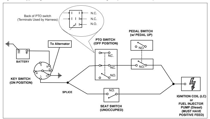
Figure 13. Typical Ignition Shutdown Linear Circuit Diagram (Liquid-Cooled and Diesel Models)
