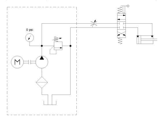
Figure 4. Needle Valve Schematic
