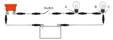
Figure 4. Series Schematic
