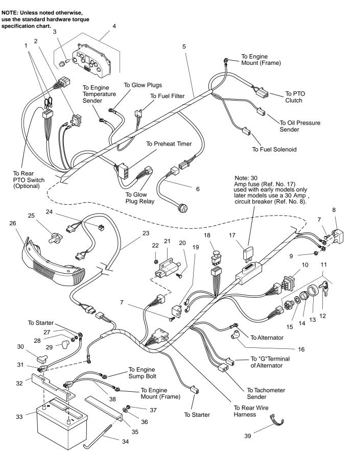
Figure 4. Exploded View Diagram – Upper Wiring Harness (Diesel Engine Models)
