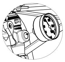
Locate the Pressure Gauge in the parts bag and thread into the open port on the manifold.
