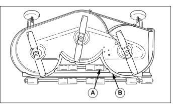
Figure 12. Anti-Scalping Rollers A. Rollers B. Mower Baffle
