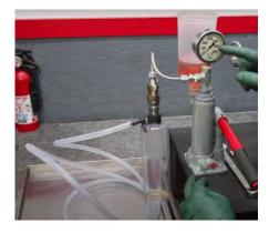
Figure 5. Fuel Injection Pressure Tester
