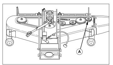
Figure 13. Idler Pulley Adjustment – 60" Decks Only A. Adjustable Idler Pulley
