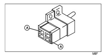
(1) Is battery voltage present at S4 park brake switch - 770 Pur and 410 Yel wires (A)?
