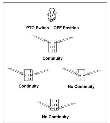
Figure 43. Test PTO Switch – OFF Position
