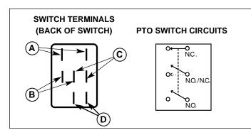
Figure 42. PTO Switch Terminals
