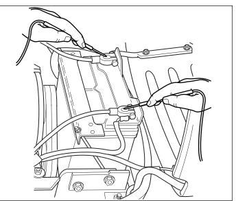
Figure 37. Check Charging Voltage
