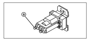
(1) Is there a minimum 14.4 ±0.5 VDC at the starter solenoid 230 Red wire connector (B)?
