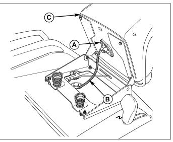
Figure 21. Seat Switch Safety System C. Seat
