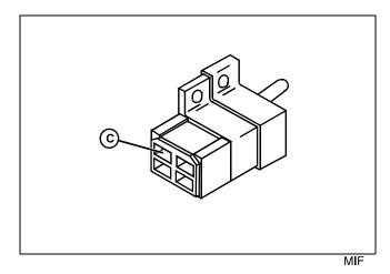
(3) Is battery voltage present at S4 park brake switch - 410 YeI wire (C)?
