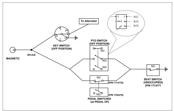
Figure 12. Typical Ignition Shutdown Linear Circuit Diagram (Air-Cooled Models)
