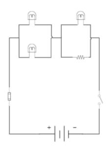
Figure 6. Series-Parallel Schematic
