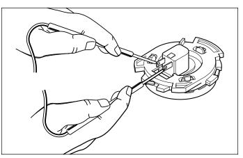
Figure 50. Test Seat Switch
