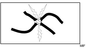
A shorted circuit may result in the wrong component operating (i.e. improper wire-to-wire contact). To test for a shorted or improperly wired circuit:
