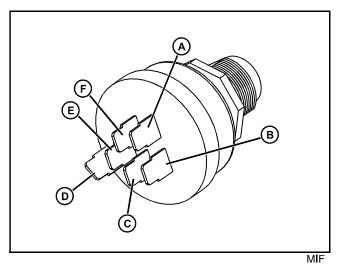
4. Use an ohmmeter to test switch continuity in OFF, RUN, and START positions.
