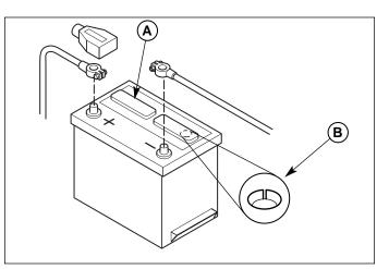
Figure 34. Check Battery ElectrolyteA. Battery CapB. Split Ring
