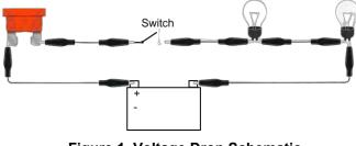
Figure 1. Voltage Drop Schematic
