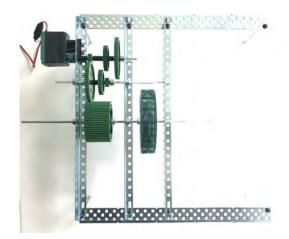
Figure 11. Completed Assembly
