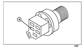
(2) Is battery voltage present at S2 key switch - 200 Red wire (A)?
