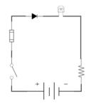
Figure1. Silicon Diode Circuit
