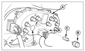
Figure 20. Instrument Panel Lamps Replacement A. Instrument Panel C. Lamp **B. Lamp Socket D.** Lamp Bezel
