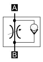
Figure 2. Flow Control Valve
