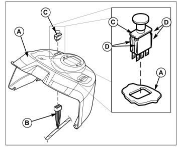
Figure 18. PTO Switch ReplacementA DashboardC. PTO SwitchB. Wire HarnessD. Locking Tabs
