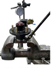
Figure 2. Hub and Dial Indicator Placement
