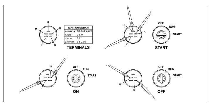
Figure 40. Ignition Switch Tests – 5-Pin Steel Body (Early Models)
