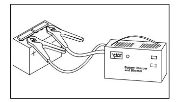
6. Connect variable rate charger to battery.
