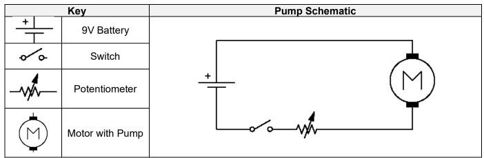
Figure 1. Electrical Schematic
