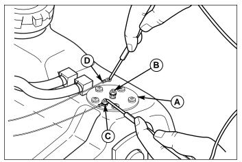
Figure 54. Fuel Level Sensor Signal TestA. SensorC. Ground TerminalB. Signal TerminalD. Signal Wire
