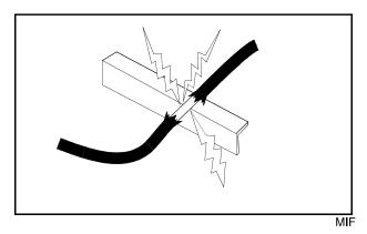
Grounded circuits usually result in no component operation or a blown fuse.
