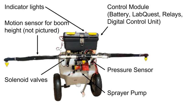
Figure 6. GPS Sprayer Trailer
