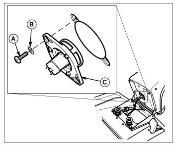
Figure 22. Seat Switch Removal and Replacement A. Screw C. Seat Switch B. Washer
