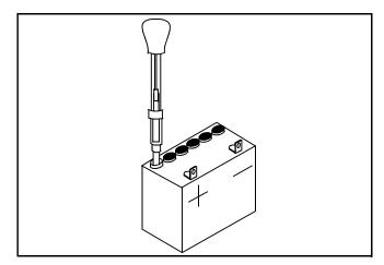
9. Use an hydrometer to check for a minimum specific gravity of 1.225 with less than 50 point variation in each cell.
