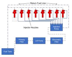
Figure 1. Diesel Fuel System
