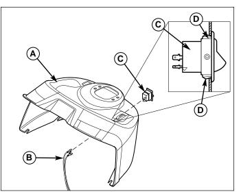
Figure 15. Headlight Switch Replacement A Dashboard C. Headlight Switch
