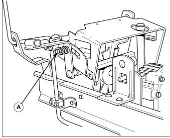
Figure 3. Cruise Control Lever Adjustment A. Tension Bolt
