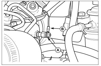
Figure 31. Seat Switch Safety System B. Sensor Wire A. Coolant Sensor
