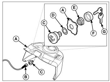
Figure 16. Ignition Key Switch Replacement
