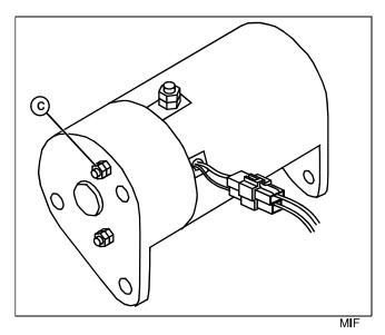
(3) Is continuity to ground present at G2 starting motor/generator - A2 terminal, 160 Blk wire (C)?
