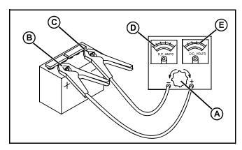
6. Turn load knob (A) counterclockwise to OFF position.
