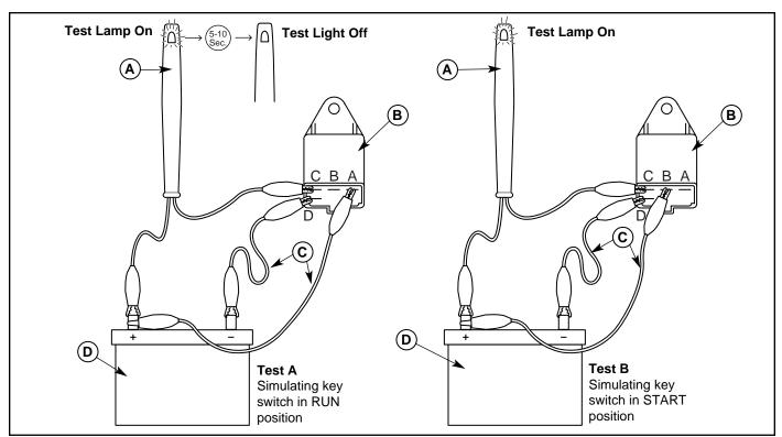
Figure 38. Testing Preheat Timer A. 12 Volt DC Lamp/Tester B. Preheat Timer
